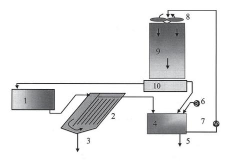
Figure 9. Simplified scheme of an aquaculture recirculation unit. 1 Growing tank; 2 Solid remover; 3 Waste discharge; 4 Pump tank; 5 Discharge; 6 Oxygen injection; 7 Water pump; 8 Spray unit; 9 Biofilter; 10 Collector tank.
